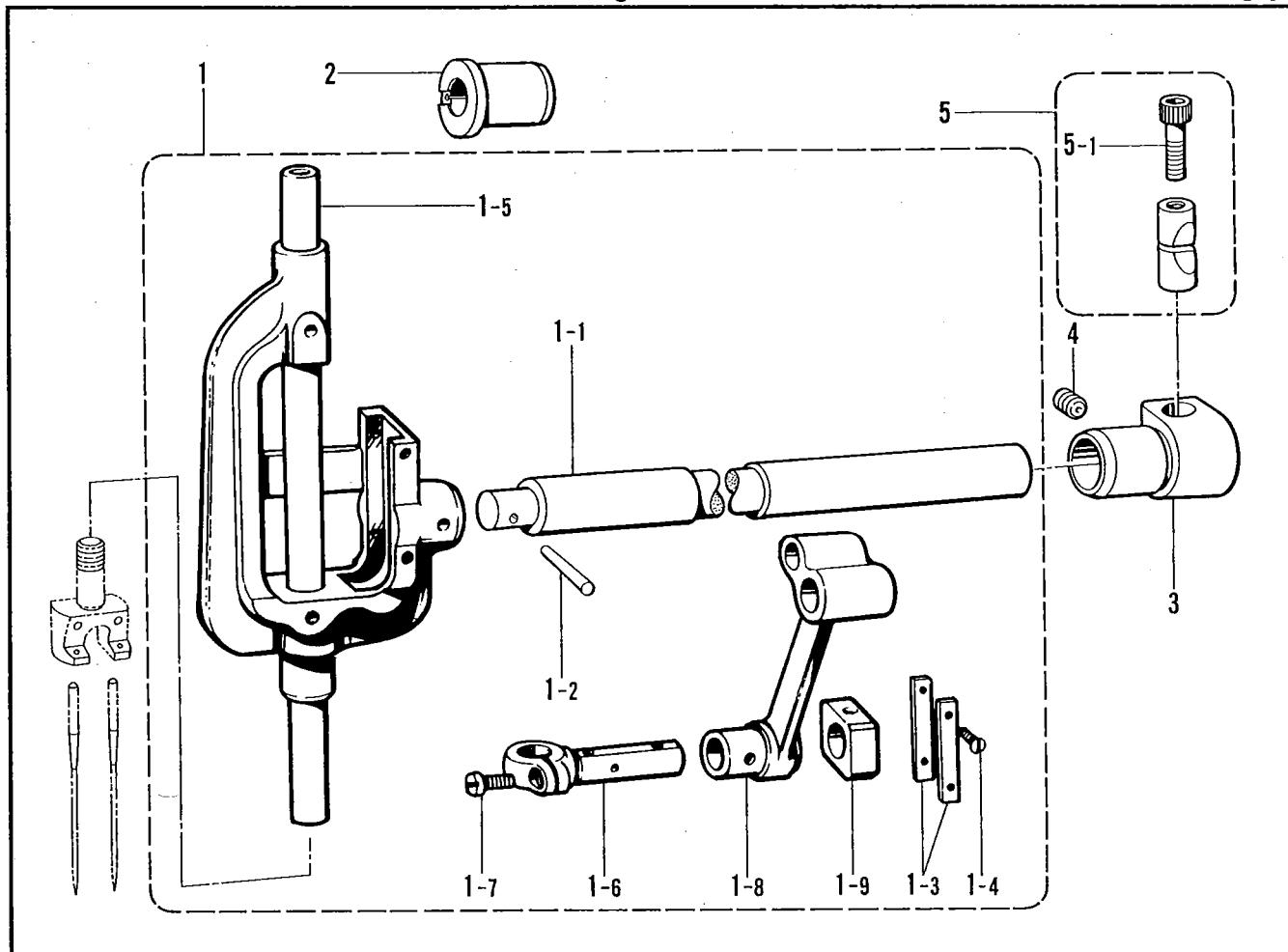
D. 下軸關係 / Lower shaft mechanism / Untere Welle /
