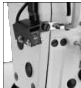
Material edge sensor (ED-2)
