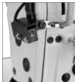
Material edge sensor (ED-2)
