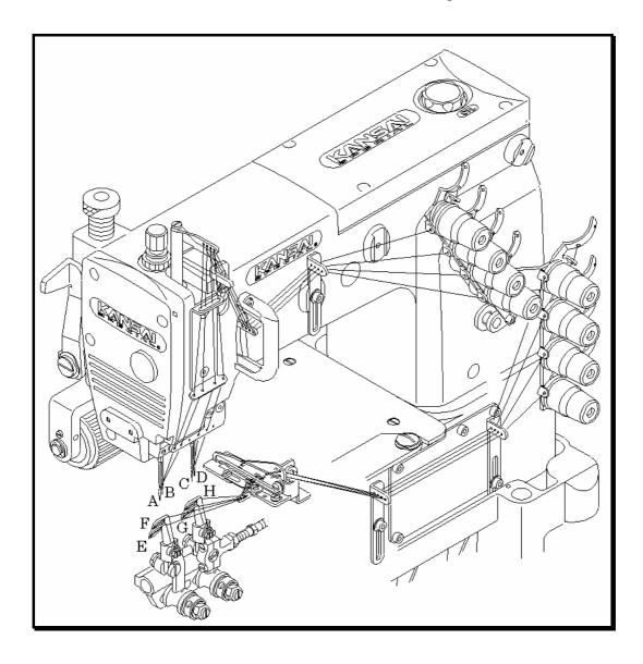
A , B , C , D  $\ldots$  Needle threads  $\qquad$  E , F , G , H  $\ldots$  Looper threads
