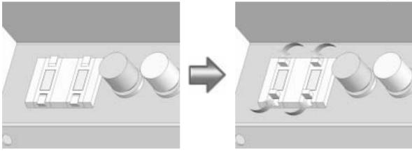
The upper push-tab switch: +1 with each pressing. The lower push-tab switch: -1 with each pressing.
