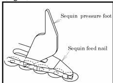
The top edge of the sequin pressure foot and the sequin feed nail shall be positioned on the center of the sequin hole. (Fig.11)
