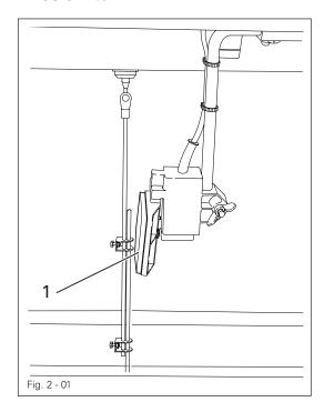
By operating knee switch 1, the presser foot can be raised when sewing is interrupted.
