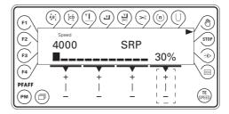
The presser foot pressure is adjusted with the sewing speed. The greater the sewing speed, the higher the pressure foot pressure. By altering the percent increase of the presser foot pressure, the increase of the presser foot pressure can be influenced by an increased sewing speed. The current pressure foot pressure can be seen on the bar graph display.
