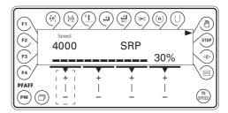
• Enter the maximum speed by pressing the corresponding +/- key.
