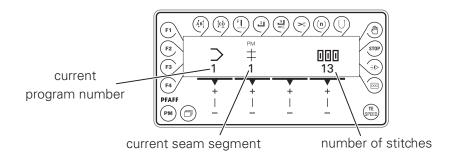
With the scroll key other menus can be selected for entering the values for start and end backtacks and the maximum speed in the corresponding seam section.
