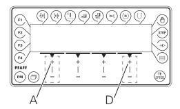
Press and hold "+" on keys A and D and switch on the machine.
