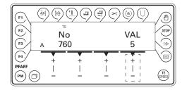
VAL Press the corresponding +/- key to set the number of remaining stitches, which can still be sewn after recognition by the bobbin thread control function.
