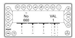
• By pressing the corresponding +/- key set the desired value for the parameter selected, e.g. "2" for the "bobbin rest thread counter on" function..
