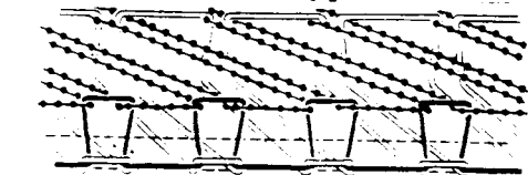
Fig.6. Stitch Formation (Stitch Type No.505)
